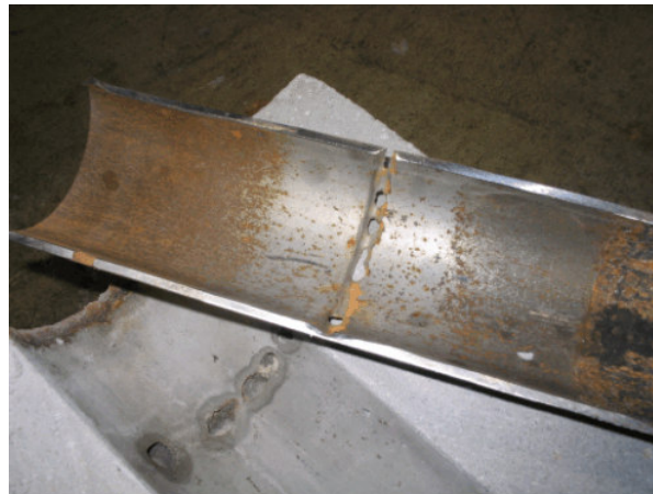
Fig 5: Slot cut into steel casing in yard test, using abrasive slurry.
